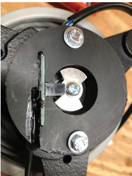
Part number. 1184071 Tachometer Horseshoe type With PP bracket
