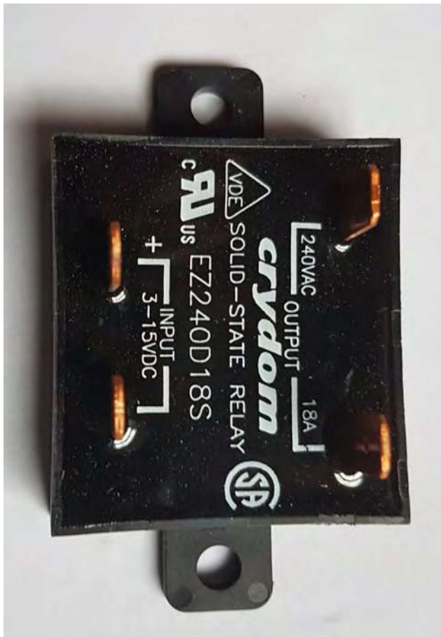
Part number. 3128002. Solid state relay 110V
